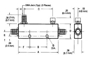
NOTE: All dimensions are  $\pm$  .020, except mounting hole diameters ( $\pm$  .005) and mounting hole location ( $\pm$  .010).
